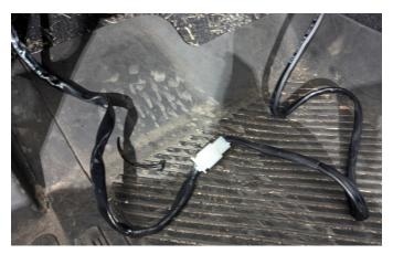
**27.** Find a suitable location for the light switch. Route the switch harness to the switch location. Pass the spade terminals out of the hole for the switch. (Optional switch panel shown)
