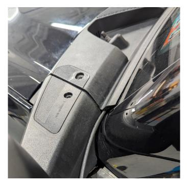
**21.** Mount the ditch light brackets using the longer M6 button-head bolts and bolt caps supplied. Tuck any excess wiring into the cowl.
