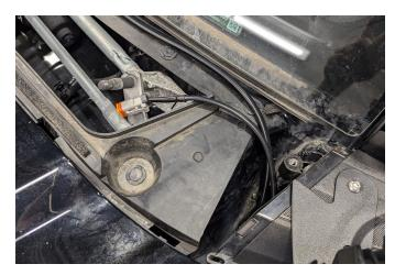
**14.** Unravel the wiring harness and locate the switch connector. Disconnect the switch harness from the wiring harness and place it off to the side for a later step.
