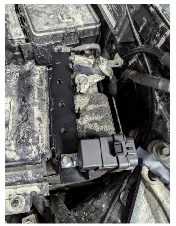
**16.** Route the pod light harnesses near the driver-side hood hinge and into the cowl. Ensure the harnesses do not get pinched when the hood is closed.
