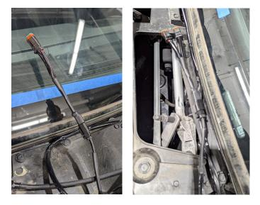
**18.** Plug the pod lights into the splitters. Tuck any excess wiring into the pocket on the driver's side of the cowl.
