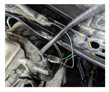
**13.** Route the upfitter harness near the driver-side hood hinge and into the cowl. Ensure the harness does not get pinched when the hood is closed.
