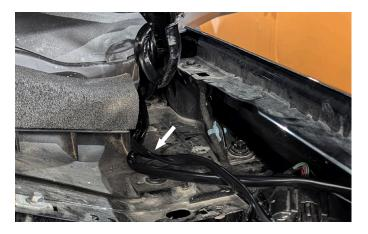
**17.** Route one of the pod light harnesses along the windshield's base over to the cowl's passenger side. Plug in one of the harness splitters. Route the other pod light harness to the driver's side of the cowl. Plug in the remaining harness splitter.
