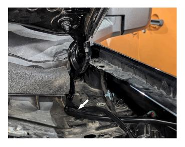
17. Route one of the pod light harnesses along the windshield's base over to the cowl's passenger side. Plug in the passenger side pod light. Route the other pod light harness to the driver's side of the cowl. Plug in the driver's side pod light. Tuck any excess wiring into the pocket on the driver's side of the cowl.
