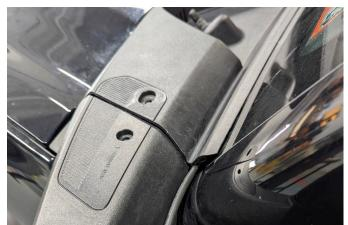
**20.** Mount the ditch light brackets using the longer M6 button-head bolts and bolt caps supplied. Tuck any excess wiring into the cowl.
