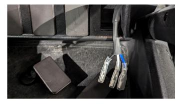
**26.** Connect the spade terminals to the switch using the included diagram. Then, press the switch into the hole until it locks in.
