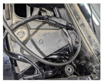
**18.** Trim the corners off the cowl cover to give the pod light wires clearance.
