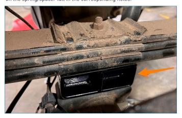
**10.** Install the supplied longer U-bolts over the leaf spring, ensuring they sit in the bracket as shown. The U-bolts should not be directly contacting the leaf springs.
