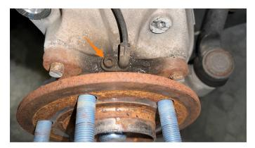
**07.** Using channel lock pliers, remove the cap from the center of the hub then use a 13mm socket to remove the axle shaft nut.
