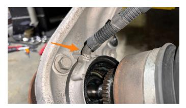
14. Let the jack down from the lower control arm. Push down on the lower control arm until the axle can be pulled from the hub. Hook the axle shaft on the sway bar end link threads to hold it out of the way. Be careful not to damage the wheel bearing seal in the hub when removing axle.
