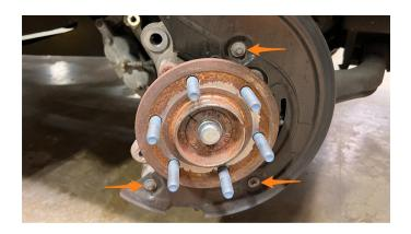
**06.** Using a 5mm allen/hex key, remove the wheel speed sensor socket head bolt and pull the sensor out.
