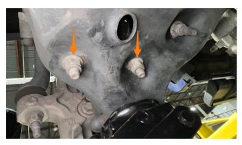
13. Remove the vacuum lines from the hub locker.
