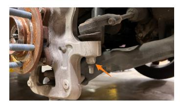
**09.** Using an 18mm wrench, remove the upper control arm ball joint nut. Counter-hold the threads using an 8mm socket. Loosely reinstall the nut so that the top of the nut is flush with the end of the threads. Using a hammer, hit the end of the threads to remove the tie rod end from the knuckle.
