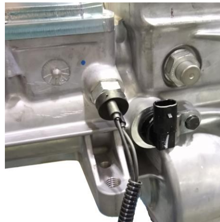
NEUTRAL SAFETY SWITCH
