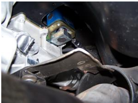
INSTALLING HORIZONTAL SHIFTER LINK CLAMP BOLTS
