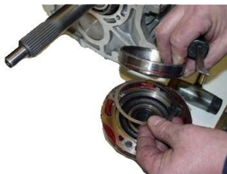
FIG. C (TKO/TKX ONLY) REMOVE BEARING RACE AND SHIMS
