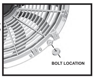
2. When mounting the Axial fan with the supplied mounting feet use the supplied rubber washer and fan spacer as shown. Use of both the spacer and washer is required to ensure the fan maintains the proper spacing.
