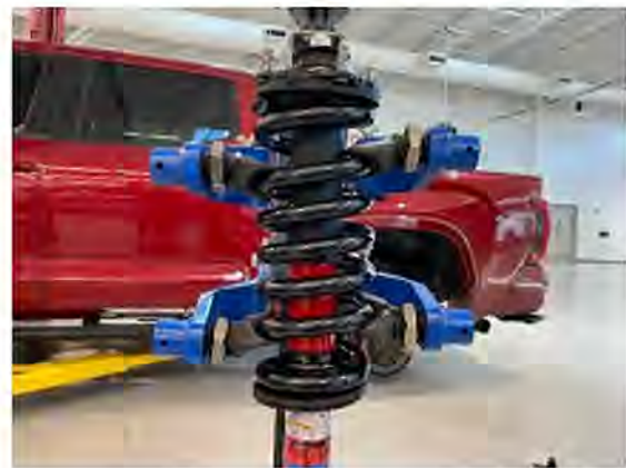
When Compressing from Mid-coil Minimum Capacity: 22,700 Nm
