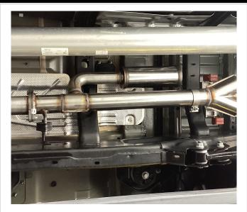
**Step 3:** Install new MagnaFlow System by loosely attaching the Resonator Assembly to the OE exhaust at the inlet flange location using the supplied fasteners and gasket.
