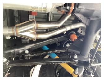
**Step 4:** Next, install the Y-Pipe Assembly by sliding it onto the Resonator Assembly and inserting both outlets onto their respective tailpipes using the OE clamp on the Passenger Side and the supplied 2.50" Clamp on the cut Driver Side. The 3.00" supplied clamp is used on the inlet.
