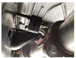
**Step 2:** To remove the exhaust, disengage the inlet flange fasteners, passenger side pipe clamp (the clamp stays attached to the OE system) and extract the hangers from rubber insulators. Do not damage or discard rubber insulators as they will be reused in the installation of the new exhaust.
