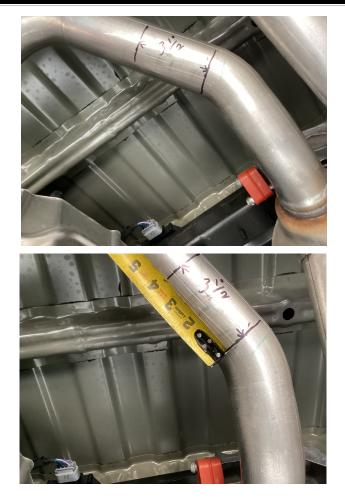
**Step 1:** To allow the removal of the OE Muffler Assembly the driver side outlet pipe must be cut. Begin by marking a cut point on the (D/S) outlet pipe 3.5" from the tangent of the second bend. Cut and deburr at this point.
