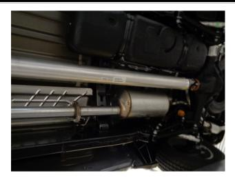
**Step 1:** Begin by removing the fasteners and gasket at the flange junction of the OE resonator,
