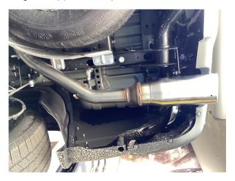
**Step 5:** Attach the Tailpipe Assemblies to the Mid Pipes using the supplied Clamps, fit the hangers into the rubber insualtors.
