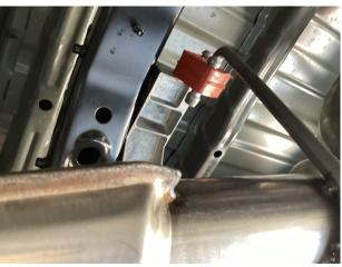
**Step 3**: Install the new system by attaching the Muffler Assembly to the OE outlet with supplied hardware and gasket. Locate the welded hangers to the rubber insulators. Leave all clamps loose for final adjustment of the complete syste once installed.
