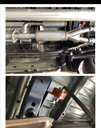
**Step 3**: Install the new system by attaching the Muffler Assembly to the OE outlet with supplied hardware and gasket. Locate the welded hangers to the rubber insulators. Leave all clamps loose for final adjustment of the complete syste once installed.
