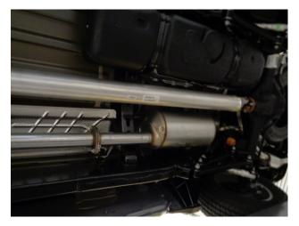
**Step 1:** Begin by removing the fasteners and gasket at the flange junction of the OE resonator,
