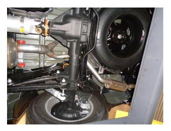
**Step 2** Working front to rear disengage all the welded hangers from the rubber insulators and remove the system. (Retain the insulators as they will be needed to mount the new MAGNAFLOW system.)
