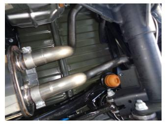
**Step 4:** Next, Loosely attach the Driver and Passenger side Mid Pipes to the Muffler Assembly using the supplied clamps
