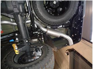
Step 1. To remove the OE exhaust system begin by unfastening the 2 bolt flange located in front of the muffler and loosening the clamp between the front and rear mufflers (over the rear axle). Working front to rear disengage the hangers from the rubber insulators and remove the exhaust. Do not damage the rubber insulators as they will be used to install the new exhaust system.
