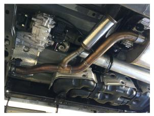
**Step 2**: Begin Installation of the new MagnaFlow system by attaching Inlet Resonator Assembly using the OE fasteners and gasket. (Leave all clamps and fasteners loose until final adjustment for fit.)
