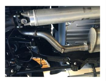
**Step4:** Next, attach the Overaxle pipe to the Muffler Assembly using the supplied 3.00" clamp and fit the hangers into the rubber insulators.
