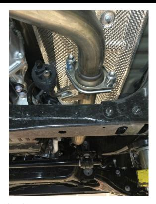
**Step 1**: To remove the OE exhaust system, remove the fasteners at the flange inlet at the front of the vehicle. Working front to rear disengage the hangers from the rubber insulators and drop the system. (Retain the Inlet fasteners, gasket and rubber insulators as they will be used to install your new system.)
