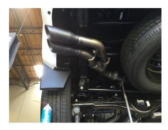
**Step 5**: Install the Tailpipe Assembly to the Over Axle Pipe fitting the hanger into the rubber Insulator.
