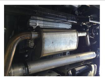
Step 3: At this point if you are installing the MagnaFlow exhaust system on a Long Bed/Double cab vehicle you will need to install the 18" Extension Pipe using the supplied 3.00" clamp. (The Short Bed/Double Cab or Long Bed/Access Cab do not require this pipe). Next install the Muffler Assembly using the supplied 3.00" clamp and fit the hangers into the rubber insulators.
