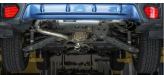
**Step 6.** Once proper positioning has been attained for the new exhaust system, tighten the clamp and mounting bolts using the torque specification on page one of these instructions. Inspect all flasteners after 25-50 miles of operation. Re-tighten if necessary.
