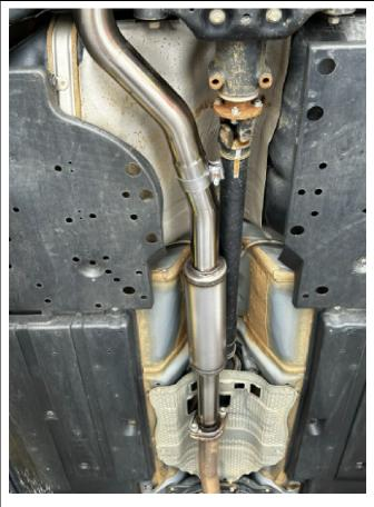
**Step 3**. Before installation of the combined center pipe, slide the Resonator Assembly into the Midpipe with the included 2.50" clamp loosely installed. Insert the hanger into the rubber insulator. Ensure the bolt holes of the flange line up to the manifold flange.
