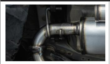
**Step 5.** Install flat gasket between Muffler and Midpipe, and insert bolts. This will position the slip fit between the Resonator and Midpipe correctly.
