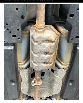
**Step 1**. Begin removal of your OEM exhaust system by unbolting the flange behind the catalytic converter and the flange connecting the Midpipe to the Muffler Assembly. Remove welded hanger from the rubber insulators. Midpipe can now be removed.
