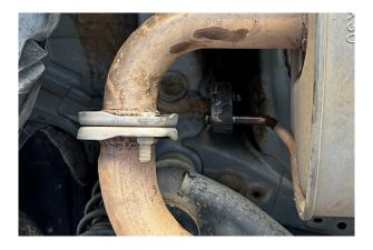
**Step 2.** Disconnect the rubber insulators that suspend the Muffler Assembly (see above). The muffler can now be removed.
