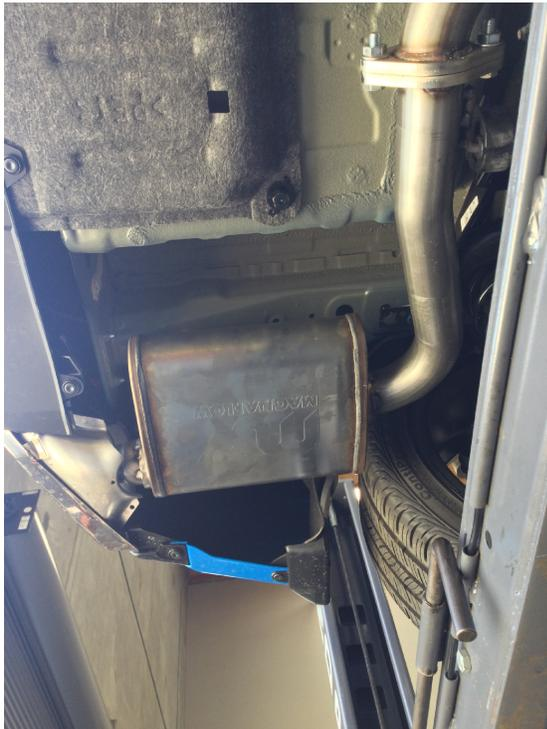
**Step 5:** Loosely attach both driver and passenger side Muffler Assembly flanges to the Y-Pipe Assembly and position the tips into the openings in the valance. Secure with the supplied gaskets and hardware. Engage welded hangers to rubber isolators.
