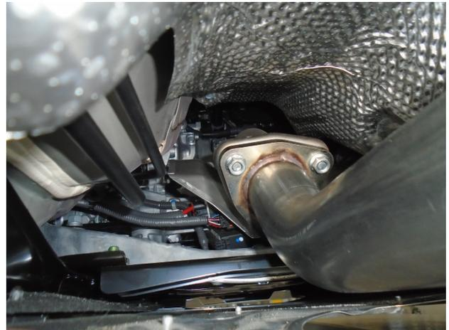
**Step 3.** Begin installation of your new MAGNAFLOW system by attaching the Inlet flange of the Inlet Resonator Assembly to the catalytic converter outlet using the OEM fasteners. Engage the welded hanger to the rubber isolator. Keep all fasteners and clamps loose until final adjustment.
