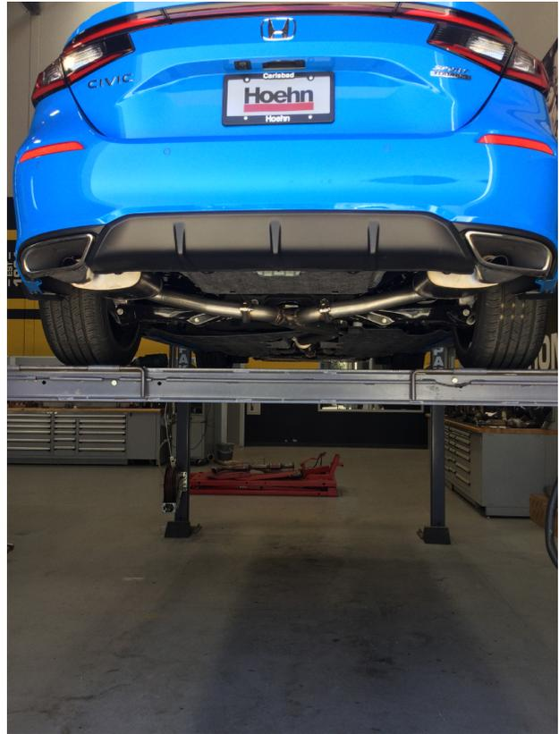
**Step 6:** Once a final position has been chosen for the new exhaust system, evenly tighten all clamps from front to rear using the torque specifications on page one of these instructions. Inspect all fasteners after 25-50 miles for operation and re-tighten if necessary.
