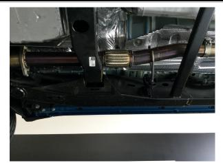
**Step 3:** Begin Installing the new MagnaFlow exhaust system by attaching the inlet pipe to the flange outlet using the OE fasteners.
