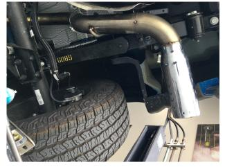
**Step 6:** Install the Tail Pipe to the Over Axle Pipe outlet using the supplied clamp. Engage the hanger to the rubber insulator.
