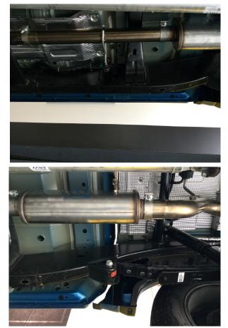
**Step 4:** Next attach the Extension pipe to the Inlet Assembly using a supplied 3.00" Clamp, fit the hanger into the rubber insulator. Next attach the Oval Muffler to the Extension Pipe with the supplied 3.00" clamp, for proper orientation the MF logo should be right side up.
