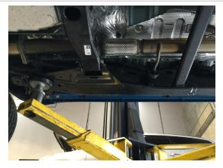
**Step 1:** Begin extracting the OE exhaust by removing the fasteners at the two bolt flange junction. Retain these fasteners to use on the new exhaust installation,
