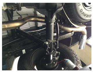
**Step 5:** Install the Over Axle Pipe to the Muffler outlet using the supplied clamp. Engage both hangers to the rubber insulators.
