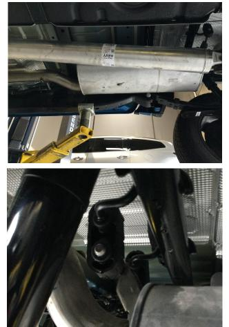
**Step 2:** Working front to rear, disengage all welded hangers from the rubber insulators and remove the system. (Retain the rubber insulators as they will be needed to mount the new MAGNAFLOW system.)
