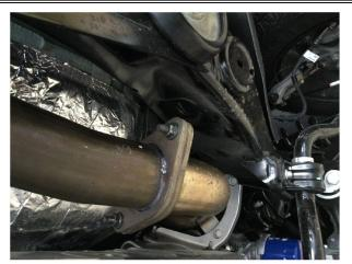
**Step 1:** To remove the OEM exhaust system, unfasten the hardware at the inlet flange (Retain the fasteners they will be used to install the new system).
