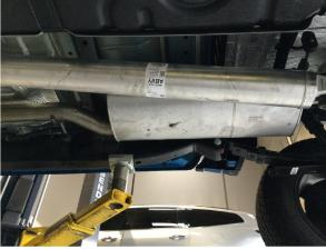
**Step 2:** Working front to rear, with the exhaust system supported, disengage all welded hangers from the rubber insulators and remove. (Retain the rubber insulators as they will be needed to mount the new MagnaFlow system.)
