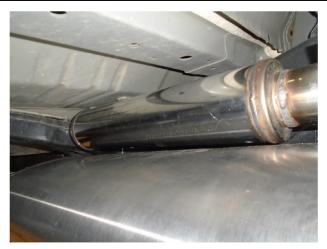
**Step 5:** When using the NDT chamber, mount it above the muffler as shown. Be sure to leave at least 1/2" of clearance between both components.
