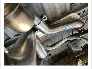
**Step 11:** Loosely install the two Mid-Pipe Assemblies using the supplied 3.00" Band Clamps. Fit the hanger into the rubbber insulator on the Driver Side Assembly.
