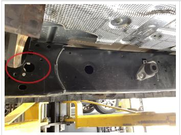
**Step 6:** At this point you will need to relocate the front hanger mount rearward from the location shown circled in red on the frame rail to the location it's currently pictured in. Add the supplied M8 Panel nuts to each hole and re-use the OE bolts.
