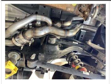
**Step 10**: Loosely Fit the X-Pipe Assembly using the supplied V-Band clamps and fitting the bypass pipe to the Mid Pipe Bypass Pipes using the supplied 2.00" clamp.
