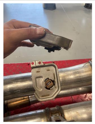
**Step 4:** Begin by removing the valve motor assembly from the OE exhaust. At this point you will need to plug the motor assembly back into the wire loom on the vehicle to reset the motor location, this is done by opening/closing the driver side door. Remove the Motor assembly, it is now ready to be installed onto the MagnaFlow valve.
