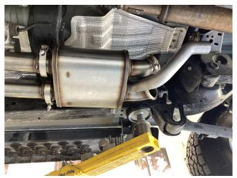
**Step 8:** Next install the Muffler Assembly by connecting the Flange Rings to the Inlet pipes with the supplied V-Band Clamps
