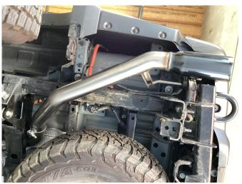
**Step 12:** Attach the Tailpipe Assemblies to the Mid-Pipe Assemblies using the supplied 3.00" clamps and ftting the hangers into rubber insulators.
