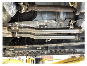
**Step 7:** Begin by installing both inlets pipes using the OE fasteners and clamp, the hanger will now fit into the relocated mount. keep all clamps and fastaners loose unit a final position has been chosen.
