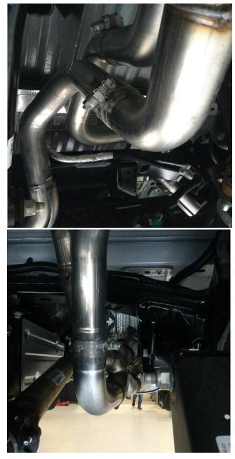
**Step 2**: Next loosen the clamps on both pipes where they pass over the rear axle. With the exhaust supported working front to back remove the OE exhaust system. You are now ready to install your new MagnaFlow exhaust system
