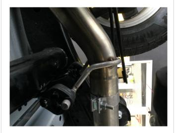
**Step 4.** Attach the Over Axle Pipe to the Muffler Assembly using the supplied 3.00" clamp and engaging the welded hangers.
