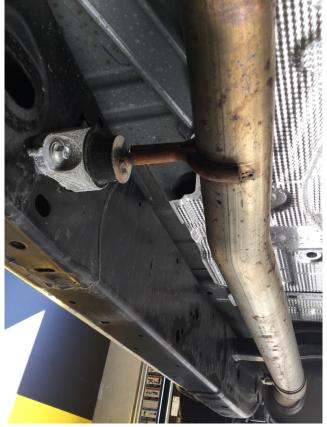
**Step 1.** To remove the OE exhaust system begin by loosening the clamps at the outlet of the catalytic converter and the inlet of the muffler. With the exhaust supported disengage the welded hangers from the rubber insulators and remove the system. Do not damage or discard the rubber insulators as they will be used to install the MagnaFlow system.
