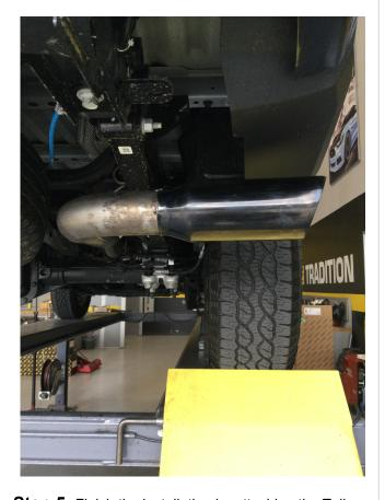
**Step 5.** Finish the installation by attaching the Tail Pipe Assembly to the Over Axle Pipes using the supplied 2.50" clamps and fitting the hanger into the rubber insulator.
