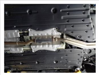
**Step 5:** Next, loosely fasten either the Resonator Assembly or the Delete Pipe to the Inlet Assembly using the supplied clamps.
