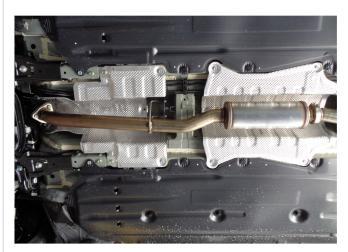
Step 4: MagnaFlow supplies this kit with a Delete pipe, it can be used in place of the Resonator for a more aggressive sound.
