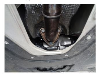
**Step 2:** To remove the OEM system first unbolt and remove the cross member at the inlet. Next, unbolt the inlet pipe at the catalytic converter flange junctions. Working front to rear disengage all welded hangers from the rubber insulators. The OE exhaust system can now be removed in one piece. Be sure to retain all mounting hardware as it will be needed to install your new MagnaFlow system
