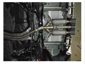
**Step 6:** Finish by loosely installing the Mid Pipe and Muffler Assembly using the supplied clamp and fitting the hangers into the rubber insulators.
