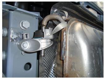
**Step 1.** To remove the OEM exhaust system begin by disengaging the grounding strip from the muffler assembly.
