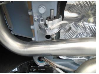
**Step 7.** Finally, clip the grounding leads to the applicable locations they were removed from.
