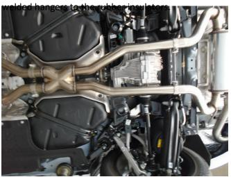
**Step 4.** Install the X-Pipe Assembly by loosely securing both inlets to the Resonator Assembly outlets using the supplied clamps. The longer pipe should be oriented on the drivers side.
