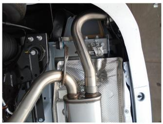
**Step 6.** At this point the installation will deviate depending on whether you have the 5.7 or 3.6L vehicle (5.7L) Install the Tail Pipe Assemblies by locating the outlets through the rear valance tip. *(3.6L) Install the Passenger Side Tailpipe and the block off pipe.* loosely secure to the Muffler Assembly outlet using the supplied clamps. Engage the welded hangers to the rubber insulators.
