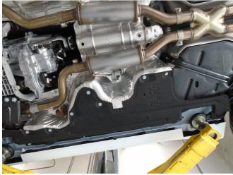
**Step 3.** Begin installing the new system by loosely attaching the Resonator Assembly inlets to the catalytic convert outlets using the supplied clamps. Engage the
