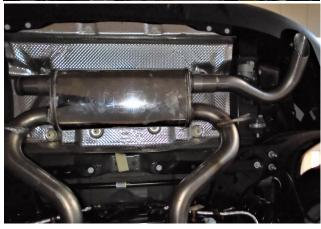
**Step 8.** Once a final position has been chosen for the new exhaust system, evenly tighten all clamps from front to rear using the torque specifications on page one of these instructions. Inspect all fasteners after 25-50 miles of operation and re-tighten if necessary.
