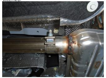
**Step 2.** Loosen the two clamps attaching the muffler assembly to the catalytic converter outlets. Disengage all welded hangers from the rubber insulator, do not discard as they will be needed to install the new MAGNAFLOW system. The OEM system can now be removed.
