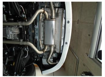
**Step 5.** Install the Muffler Assembly by loosely attaching the two inlet pipes to the X-Pipe Assembly outlet pipes using the supplied clamps. Engage the welded hangers to the rubber insulators.
