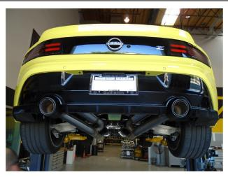
**Step 7:** Once a final position has been chosen for the new exhaust system, evenly tighten all clamps from front to rear using the torque specifications on page one of these instructions. Inspect all fasteners after 25-50 miles for operation and re-tighten if necessary.
