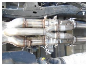
**Step 13:** loosely Fit the X-Pipe Assembly using the supplied 3.00" clamps and fitting the bypass pipe to the Mid Pipe Bypass Pipes using the supplied 2.00" clamps.
