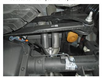
**Step 2:** Next loosen the clamps on both pipes where they pass over the rear axle. With the exhaust supported working front to back remove the OE exhaust system. You will also need to remove the spare tire to install this system. You are now ready to install your new MAGNAFLOW exhaust system
