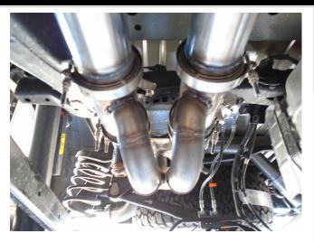
**Step 11**: Loosely install the two Mid-Pipe Assemblies using the supplied clamps. Orientate as shown
