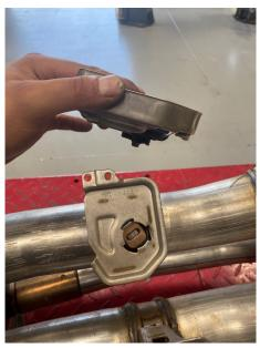
**Step 4:** Begin by removing the valve motor assembly from the OE exhaust. At this point you will need to plug the motor assembly back into the wire loom on the vehicle to reset the motor location, this is done by opening/closing the driver side door. Remove the Motor assembly, it is now ready to be installed onto the MagnaFlow valve.
