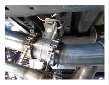
**Step 12:** Next install the valves using the supplied clamps and fit the electrical plugs.
