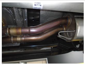
**Step 1:** Begin removal of your OE system by first loosening the clamps in front of the muffler assembly and un-plugging the electrical connections to the valves. Disengage all welded hangers from the rubber insulators. Retain the large slide clamp and rubber insulators as they will be used to install your new system.
