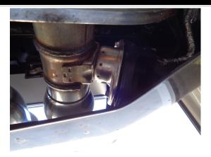
**Step 2.** Next if you have rear OE exhaust valves you will need to unplug the electrical connection on the rear Exhaust Valve Control Motors (Qty 2) located on the OEM exhaust assembly.
