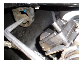
**Step 5.** If your vehicle has valves re-connect the wiring harness plugs to the Valve motors, re-install the rear valance.
