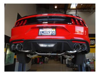
**Step 6**. Once a final position has been chosen for the new exhaust system, evenly tighten all clamps and fasteners using the torque specifications on page one of the instructions. Inspect all fasteners after 25-50 miles of operation and re-tighten as necessary.
