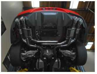
**Step 5**. Finish by installing the NDT Resonator Assemblies using the suppled 2.50" V clamps and rotating so they are level or horizontal to the ground. It is critical that the NDT Resonators are not in close proximity to moving suspension, plastics, or electronics as they can get extremely hot.
