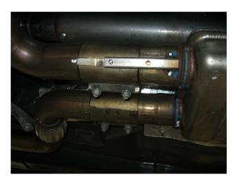
**Step 1.** Remove the OE exhaust system by first loosening the clamps located in front of the resonator. Next working front to rear extract the hangers from the rubber insulators and remove the complete exhaust system. Retain insulators and clamps as they will be used to install the new system.
