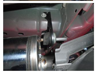
**Step 4**. Next install the passenger side NDT Muffler Assembly followed by the driver side NDT Muffler Assembly using supplied 3.00 Band Clamps and engaging the hangers into the rubber insulators.
