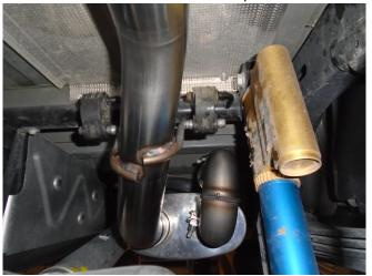
Install the Over Axle Pipe to the Muffler outlet using the supplied clamp. Engage both hangers to the OE rubber insulators.
