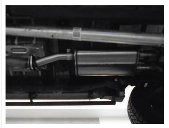
**Step 5:** Next attach the Oval Muffler to the Inlet Pipe with the supplied 2.50" clamp. This exhaust system is configured to allow the user to tune the sound. For a more moderate exhaust sound install the U-pipe Assy and the 4.00" NDT Chamber (as shown) using the suppled 2.50" clamps. For a more aggressive sound see configuration chart below.
