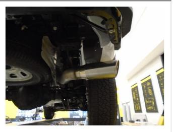
**Step 5.** Finish by installing the Tail Pipe Assembly to the over axle Resonator assembly using the supplied 4.00" clamp, fitting the welded hanger into the rubber insulator.
