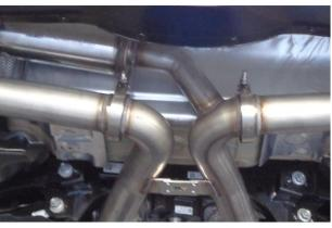
**Step 4.** Next install the passenger side Extension/Resonator Assembly followed by the driver side Extension pipe using supplied V-Clamps.
