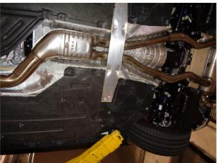
**Step 1.** To remove the OEM system first unplug the electrical connector at the exhaust valve located on the passenger side Tail Pipe. Begin by removing the cross brace then unbolt the mounting bracket and loosen the clamp at the exhaust inlet. Remove all welded hangers from the rubber insulators and remove the exhaust. Do not damage the fasteners or rubber insulators as they will be used to install the new MagnaFlow system.
