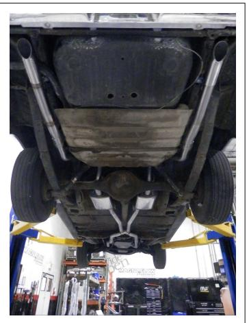
**Step 3.** Once a final position has been chosen for the new exhaust system, evenly tighten all clamps from front to rear using the torque specifications on page one of the instructions. Inspect all fasteners after 25-50 miles of operation and re-tighten if necessary.
