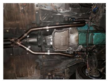
**Step 2.** Loosely attach the inlet of each Manifold Pipe to the OEM Manifold using the supplied gaskets and hardware. Then attach both Manifold Pipes outlets the the inlet end on Magnaflow System #19303 using the supplied clamps.
