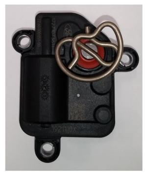
**Step 2.** If the spring becomes dislodged, reinstall in the orientation seen above. A replacement spring has been supplied in case the OE part is damged.
