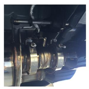
**Step 4.** When installing the valves orient them to be free of any interferences like the body, exhaust system or hangers that can damage it. Once a final position has been chosen for the new valves, evenly tighten all the clamps from front to rear. Re-connect the wiring harness plug to the Valve motors and wire mounting bracket. Inspect all fasteners after 25-50 miles of operation and retighten if necessary.
