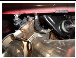
**Step 1.** Unplug the electrical connection on the Exhaust Valve Control Motors (Qty 2) located on the OE exhaust assembly, also disconnect the wire harness mounting plug.
