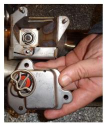
**Step 3.** Remove the valve delete pipes from the MagnaFlow system. If needed, use the supplied clamps when installing the new valves. Before mounting the new valve bodies to the exhaust system the motors will need to be transferred onto the new valve. First place the Actuator Shield on top of the valve and using supplied hardware install the OE motor to the new Magnaflow valve locking the spring into place using the OEM specified torque.
