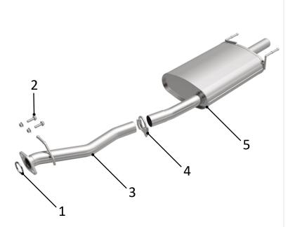
(Carefully read all instructions before installation) Disconnect the vehicle's battery before removal of the OEM exhaust system. This will prevent electrical accidents and will reset the computer if it applies to the vehicle. Remove existing exhaust system from the vehicle. Only remove parts that will be replaced. Clean existing flange with a wire brush to ensure proper sealing.
