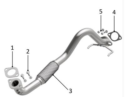
(Carefully read all instructions before installation) Disconnect the vehicle's battery before removal of the OEM exhaust system. This will prevent electrical accidents and will reset the computer if it applies to the vehicle. Remove existing front pipe from the vehicle. Only remove parts that will be replaced. Clean existing flange with a wire brush to ensure proper sealing.
