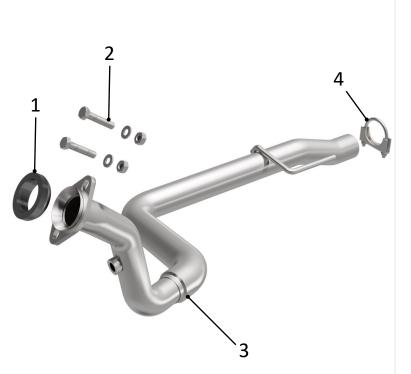
(Carefully read all instructions before installation) Disconnect the vehicle's battery before removal of the OEM exhaust system. This will prevent electrical accidents and will reset the computer if it applies to the vehicle. Remove existing front pipe from the vehicle. Only remove parts that will be replaced. Clean existing flange with a wire brush to ensure proper sealing.
