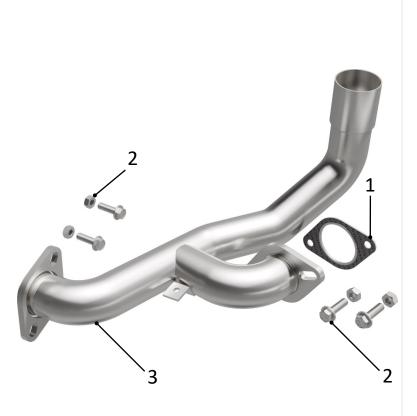
(Carefully read all instructions before installation) Disconnect the vehicle's battery before removal of the OEM exhaust system. This will prevent electrical accidents and will reset the computer if it applies to the vehicle. Remove existing front pipe from the vehicle. Only remove parts that will be replaced. Clean existing flange with a wire brush to ensure proper sealing.
