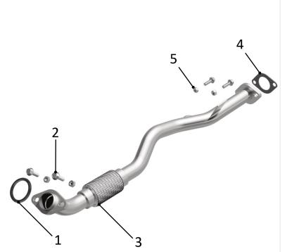
(Carefully read all instructions before installation) Disconnect the vehicle's battery before removal of the OEM exhaust system. This will prevent electrical accidents and will reset the computer if it applies to the vehicle. Remove existing front pipe from the vehicle. Only remove parts that will be replaced. Clean existing flange with a wire brush to ensure proper sealing.
