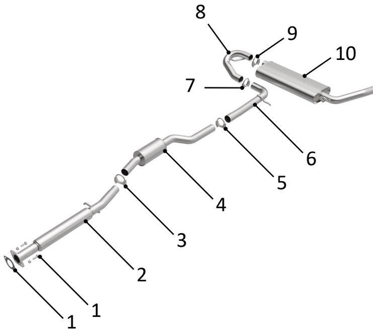
**STEP 1:** (Carefully read all instructions before installation) Disconnect the vehicle's battery before removal of the OEM exhaust system. This will prevent electrical accidents and will reset the computer if it applies to the vehicle. Remove existing exhaust system from the vehicle. Only remove parts that will be replaced. Clean existing flange with a wire brush to ensure proper sealing.
