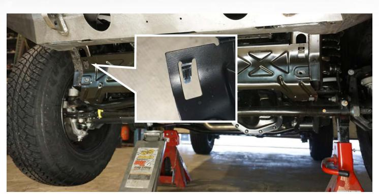
First remove the crash bar, there are two bolts holding it on.
