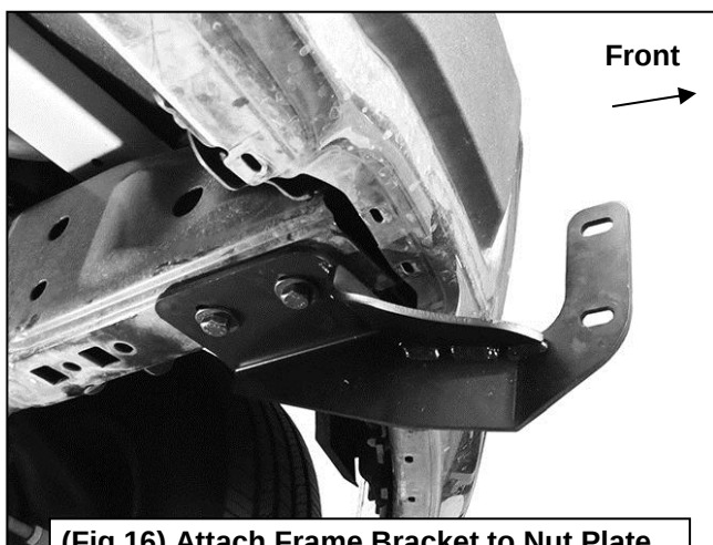
(Fig 16) Attach Frame Bracket to Nut Plate.
