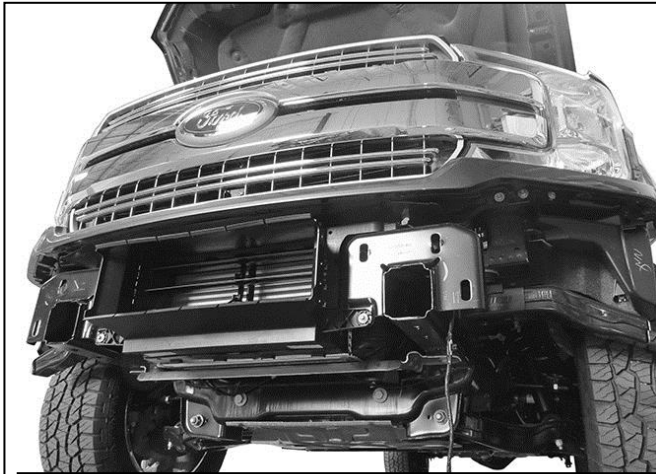
(Fig 18) 2018 models: Remove bumper assembly
