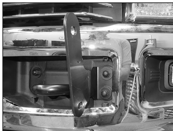
(Fig 6) Reuse factory bumper bolts to attach driver/left Frame Bracket to bumper
