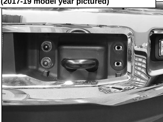
(Fig 3) Remove outer bumper bolts only
