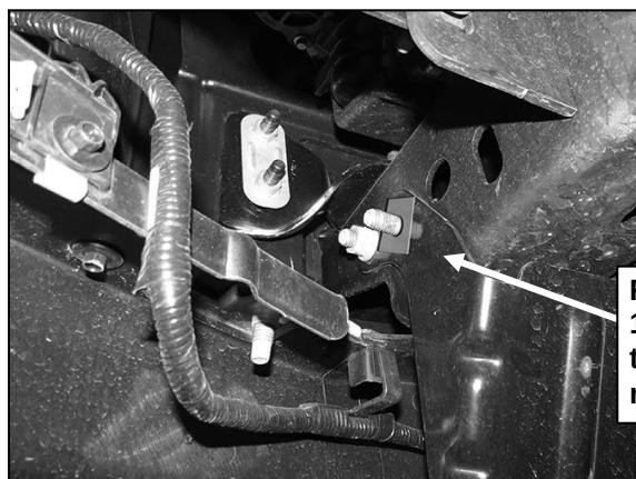
(Fig 10) Driver/left frame extension pictured
