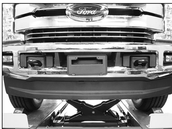
(Fig 7) Remove plastic air dam from bumper
