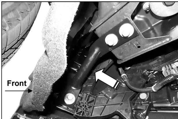
(Fig 7) Turbo Charged (gas and diesel models) with tow hooks only. Remove outer bumper supports (arrow)
