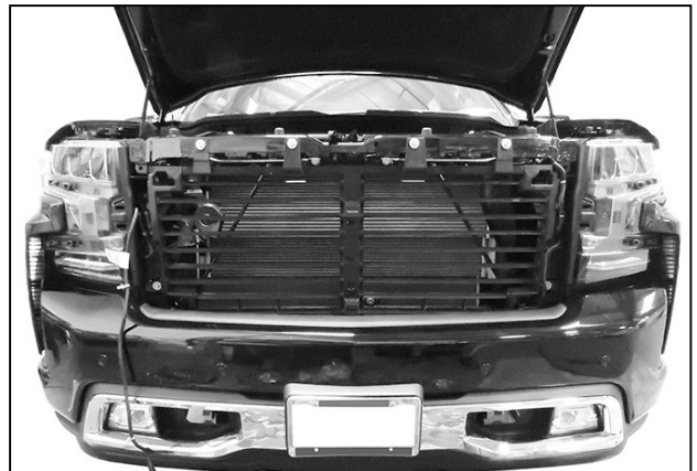
(Fig 6) Turbo Charged (gas and diesel models) with tow hooks only. Firmly pull grille straight out from vehicle
