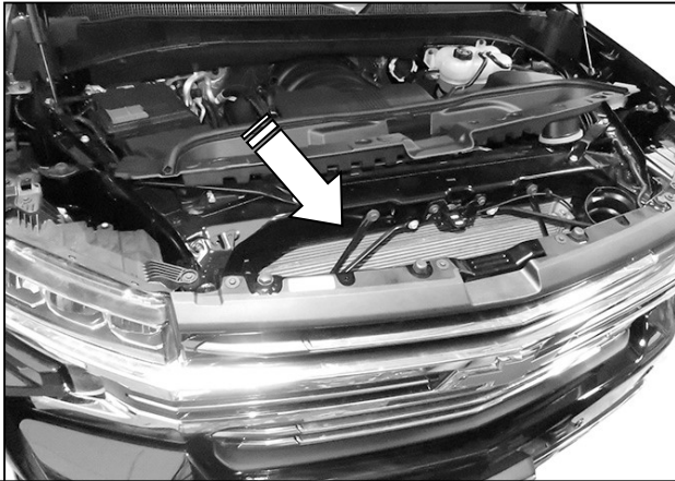
(Fig 5) Turbo Charged (gas and diesel models) with tow hooks only. Remove cover from top of radiator and grille, (arrow), Remove screws/hardware attaching grille and pull grille to release clips
