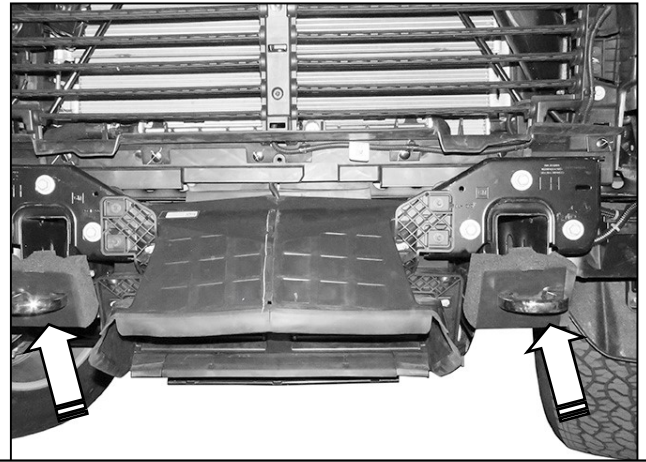
(Fig 11) Turbo Charged (gas and diesel models) with tow hooks only. Partially remove the shutter assembly to remove tow hooks and hardware (arrows)
