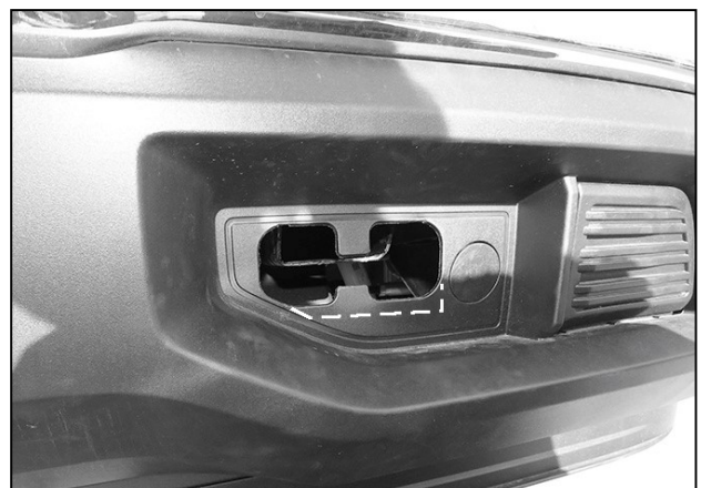
(Fig 4) Tow hook removed. Bottom of opening may need to be trimmed to clear the Mounting Bracket
