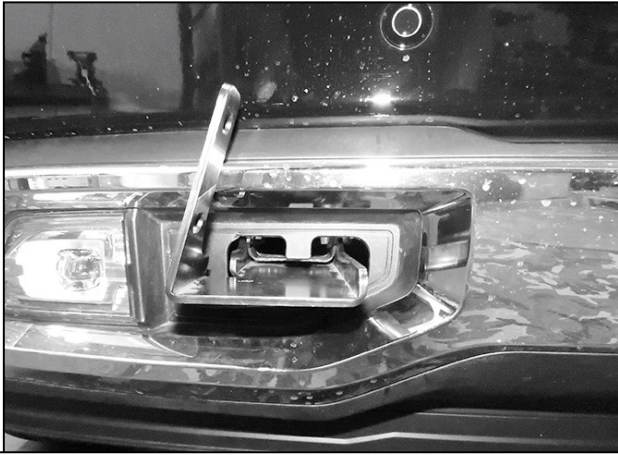
(Fig 14) Passenger/right Bracket installed
