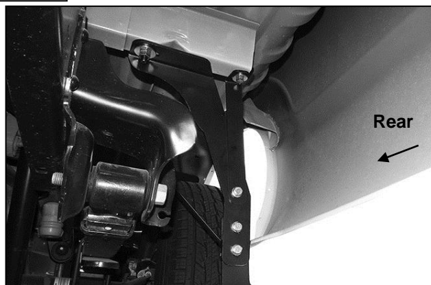
(Fig 12B) 1999-2010 Complete driver side bed Mounting Bracket assembly pictured
