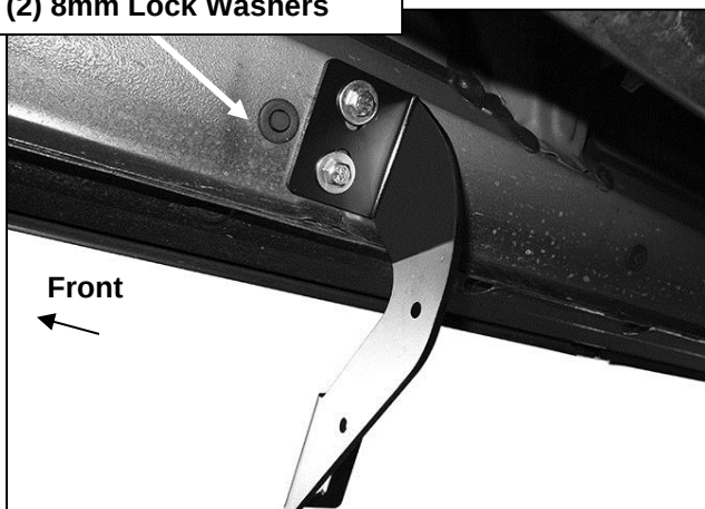
(Fig 7) Passenger side center Bracket installation
