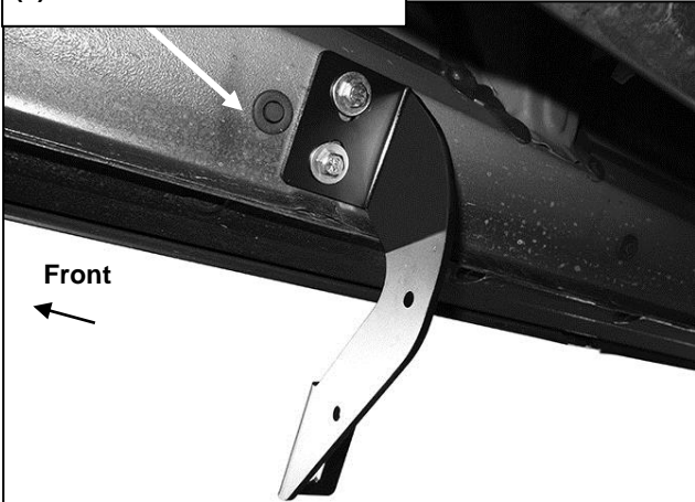
(Fig 7) Passenger side center Bracket installation
