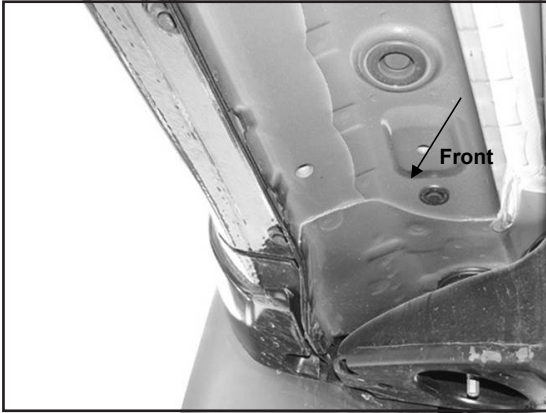
(Figure 1) Attach Passenger/Right Front Mounting Bracket to Passenger/Right Front mounting location using threaded inserts.
