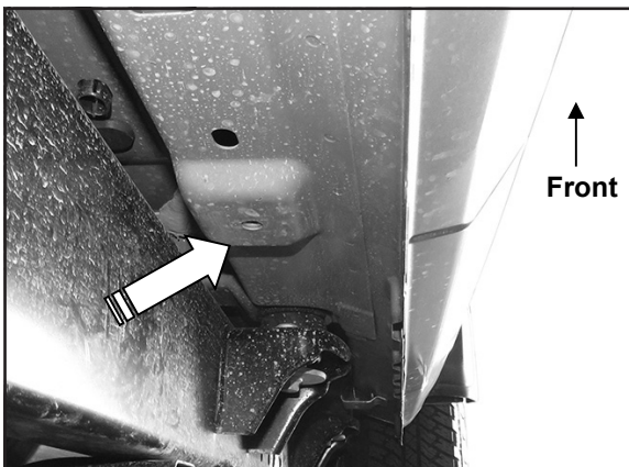
(Figure 5) Driver/left center mounting location.
