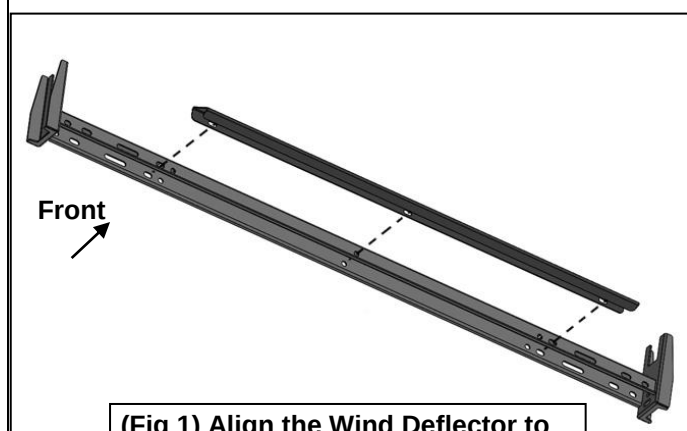
(Fig 1) Align the Wind Deflector to the front face of the Cross member
