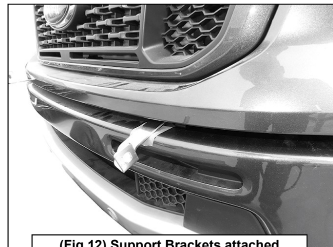
(Fig 12) Support Brackets attached
