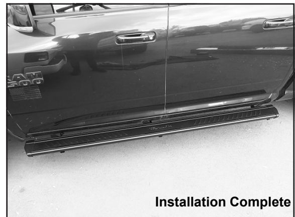
(Figure 24) Attach the driver/left Running Board to the center and rear Brackets.
