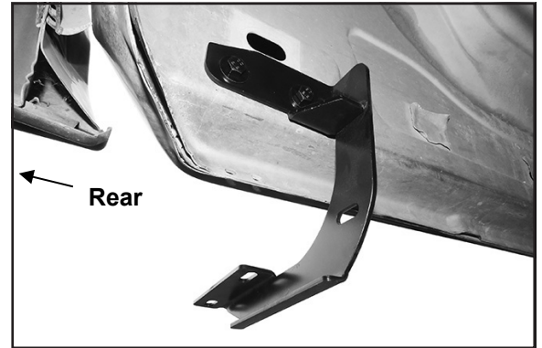
(Figure 20) Driver/left rear Bracket installed.
