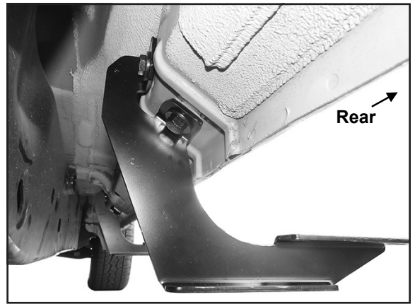
(Figure 8) Center/Rear Bracket attached to the passenger/right rear mounting location.
